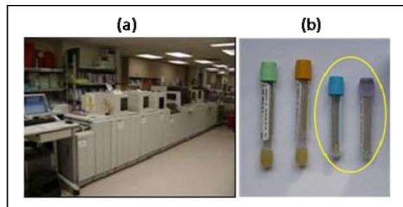
**Figure 9: (a) The Modular Pre-Analytics machine (MPA); (b) Blue and purple capped stat specimen that should not be sent through the MPA.**
