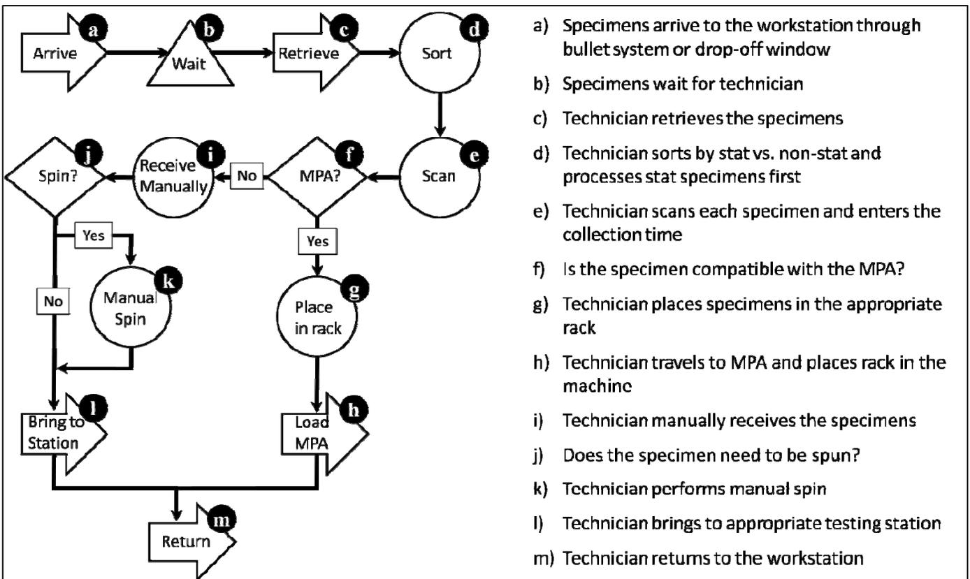
**Figure 5: Process flow diagram of the workstation**
